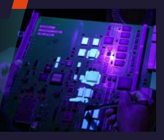
The UV Light Booth is a powerful inspection tool designed to reveal discrepancies, contamination, and process issues with precision using UV light.
