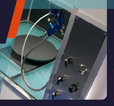
The SB2900 is expertly designed for precise batch spraying of conformal coatings onto Printed Circuit Assemblies (PCAs). Engineered for maximum efficiency and ease of use, it enhances operator control while reducing overspray and material waste.
