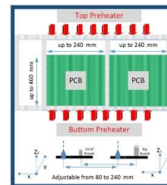
Novo™ 460PD flux, preheat and soldering configuration
