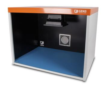
An anti-static mat complete with antistatic earthing points is supplied fitted to the work base, and an exhaust spigot is located centrally to the rear panel for connection to an external exhaust duct. The spigot measures 25 x 80 mm in diameter.
