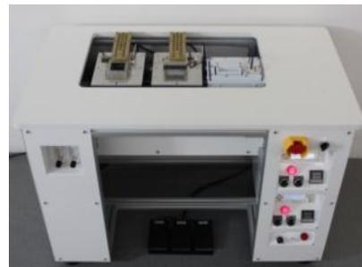
The solder, flux stations and controls are easily accessed.
