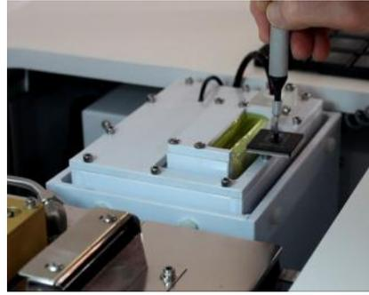
Fluxing fine pitch QFPs with "Side Wave"...
